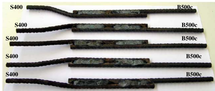
Fig. 11 Compressive failure of welded of S400 corroded specimens welded to B500 c noncorroded bars
