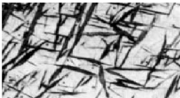
Fig. 2 Martensite particles in a steel. Microscopic inner structure of martensite
