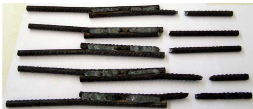
Fig. 6 Illustration of the tensile mode of failure of welded specimens
